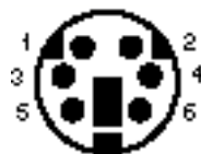
Figure 3-3: Serial Port Connector - External Pin Locations
