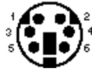
Figure 4-1: Serial Port Pin Locations
